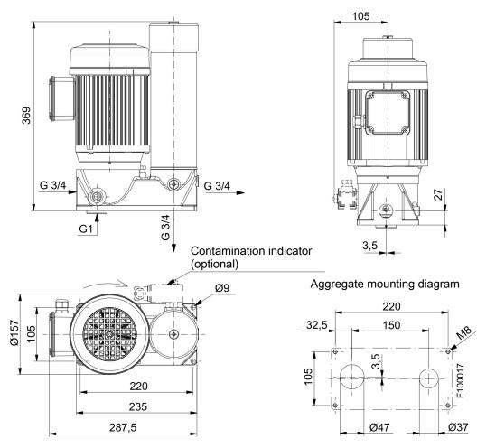
**Note:** When installing next to the oil reservoir please not the intake! When determining the bores on the reservoir be sure the contamination indicators remains visible!
